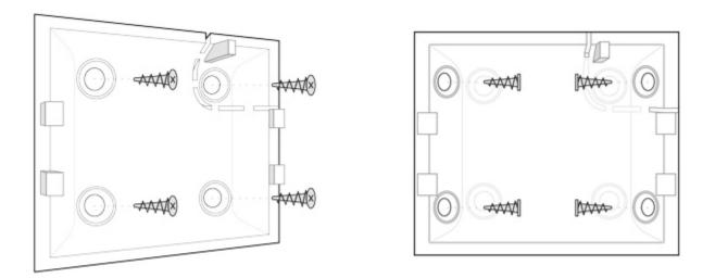
Attach the SmartBracket panel to the surface using bundled screws, using at least two fixing points (one of them – above the tamper). After selecting other attachment screws, make sure that they do not damage or deform the panel. If the LED indicator of the detector is not actuated after installation in SmartBracket, check the status of the tamper in the **Ajax Security System application** and then the fixing tightness of the panel.
